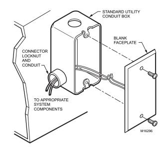
Fig. 2. Mounting, wiring for C7772.
